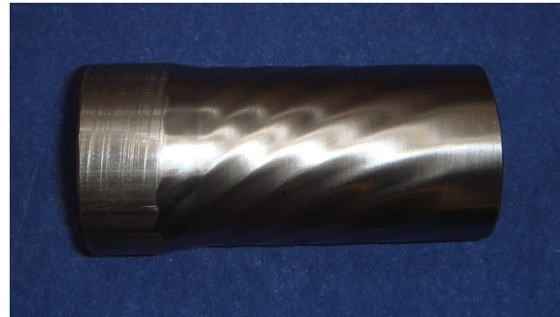
Failure during reduction
